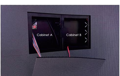
In order to make it seamless assembly between adjacent cabinets, we designed one module to cross 2 cabinets, which is perfect for curved LED screens.
